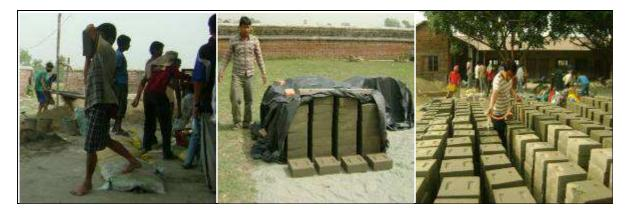
Figure 14 Carrying, storing and water curing of CSEB
