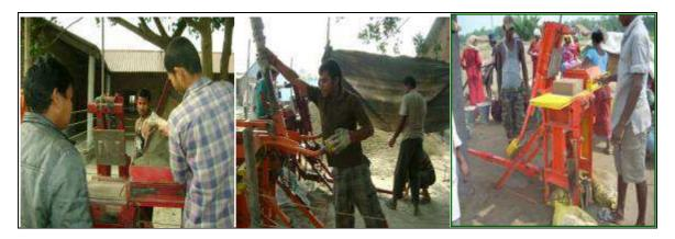
Figure 13 Pouring mixed soil, handling machine and CSEB production at Morang district
