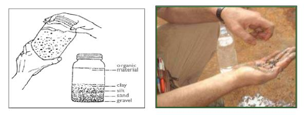
Figure 9 sedimentation test carried at Morang district
